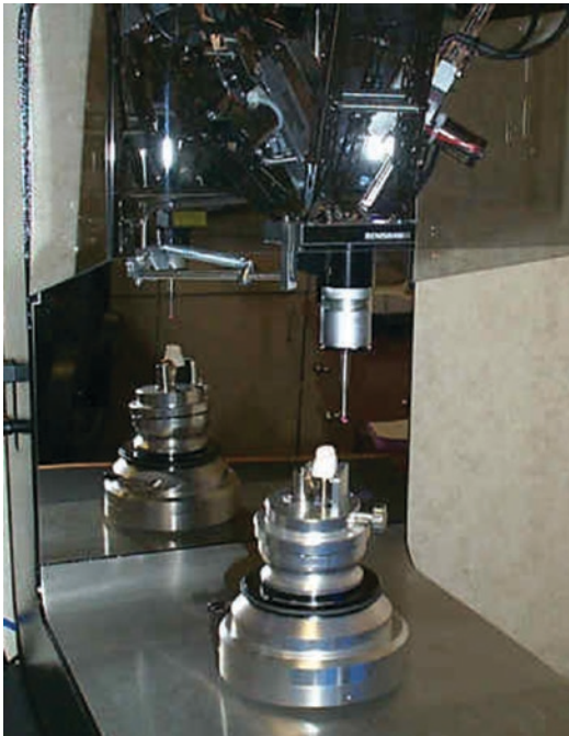
Fig. 1.6 Former contact scanners. Procera® by Nobel Biocare
