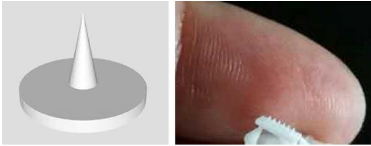
FIGURE 54.8 SLA printed high-resolution microneedles.
