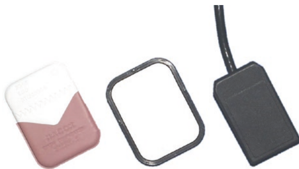
Fig. 2.4 An example of the different types of receptors in dental radiography. An E-speed film (left), a photostimulable plate (middle), and a charge-coupled device (right)
