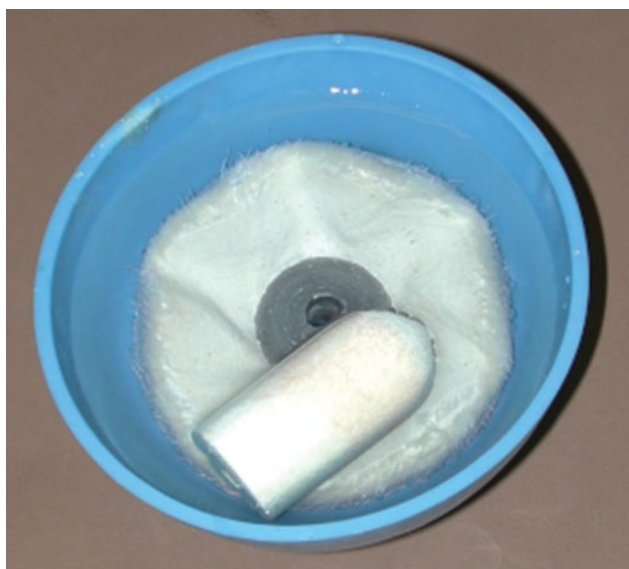
Figure 27.12 Use wet felt cones on a lathe to polish the external surfaces up to the peripheral fold.
