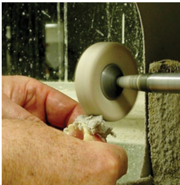
Figure 27.11 Use wet rag wheels mounted on a lathe to polish the external surfaces up to the peripheral fold.
