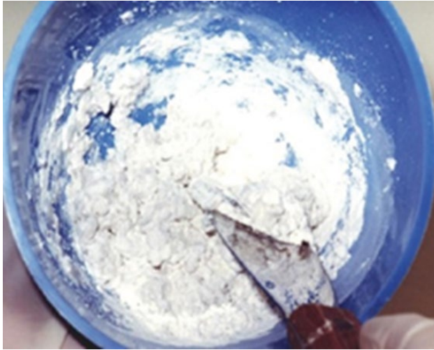
Figure 2.8 Use a round-edged flexible spatula to vigorously mix gypsum powder with water to incorporate it into a homogenous mixture.
