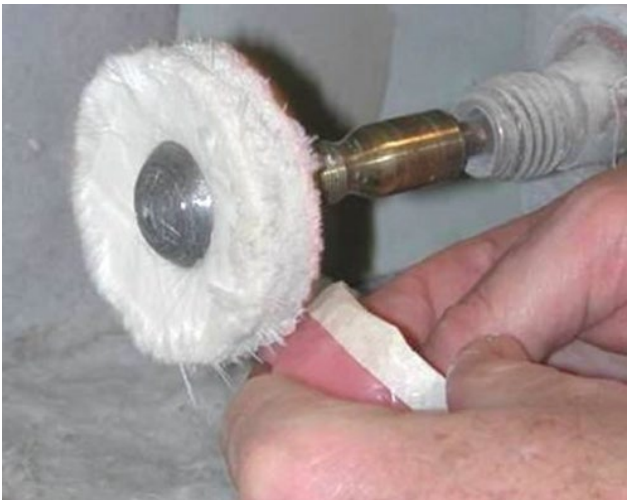
Figure 27.16 Place a piece of masking tape over the teeth to prevent inadvertent abrading of their surfaces.
