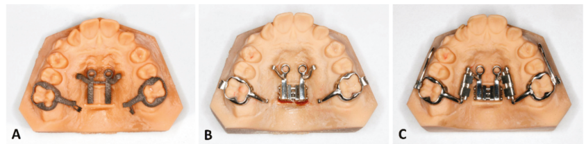
Figure 6. Post-processing of a 3D-printed appliance. (A) Unprocessed printed parts, (B) surface milled and polished, Jack screw and tubes welded to the appliance, (C) completed appliance for molar distalization and simultaneous face mask wear (hooks).
