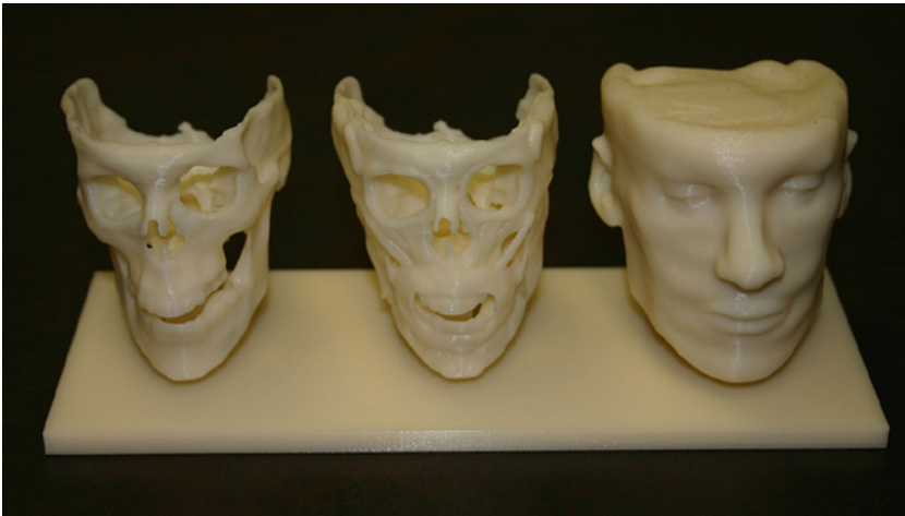
Figure 3.5 Example of the irregular organic shapes that are best fabricated using additive manufacturing techniques.
