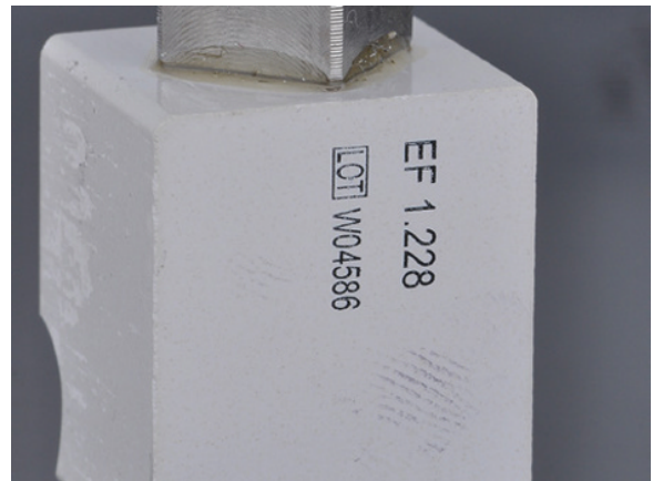
Figure 5.22 Enlargement factor is usually provided by the manufacturer or pre-programmed in the milling system.
