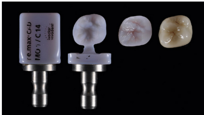
Figure 5.21 Lithium disilicate ceramic block: milled restoration, external stain, and glaze application, fully crystallized restoration (from left to right).
