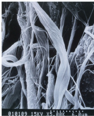
Fig 4-32 SEM image of Someya's sinew string rich in collagen (courtesy of Department of Anatomy, Tokyo Dental College).
