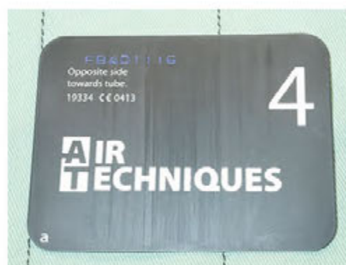
Figure 1.9 Computed radiography (CR) Size 4 image sensor: indirect plate. Source: Courtesy of Chad Lothamer, DVM, DAVDC, University of Tennessee College of Veterinary Medicine.
