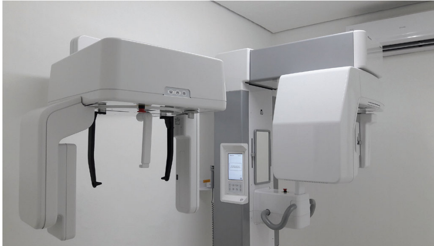
Figure 2.1 A CBCT device integrated with cephalometric and panoramic radiographic functions (Cranex® 3D, Soredex, Tuusula, Finland).
