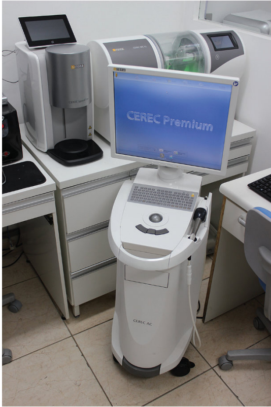
Figure 2.7 The CEREC Omnicam intraoral scanner integrated with a milling device from the same manufacturer (Dentsply Sirona).
