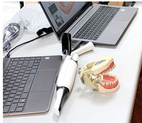
Figure 2.6 The TRIOS® 4 intraoral scanner (3Shape A/S), which uses confocal technology and enables integration with CAD software programs and CAM devices from other manufacturers.
