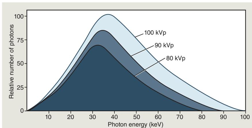
**Fig. 1.17** Spectrum of photon energies generated in an x-ray machine showing that as the kVp is increased (mA and s held constant), there is a corresponding increase in the mean energy of the beam, the total number of photons emitted, and the maximal energy of the photons. Compare with Figs. 1.15 and 1.16.
