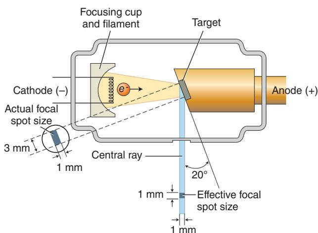
**Fig. 1.8** The angle of the target to the central ray of the x-ray beam has a strong influence on the apparent size of the focal spot. The projected effective focal spot (seen below the target) is much smaller than the actual focal spot size (projected to the left). This provides a beam that has a small effective focal spot size to produce images with high resolution, while allowing for heat generated at the anode to be dissipated over the larger area.
