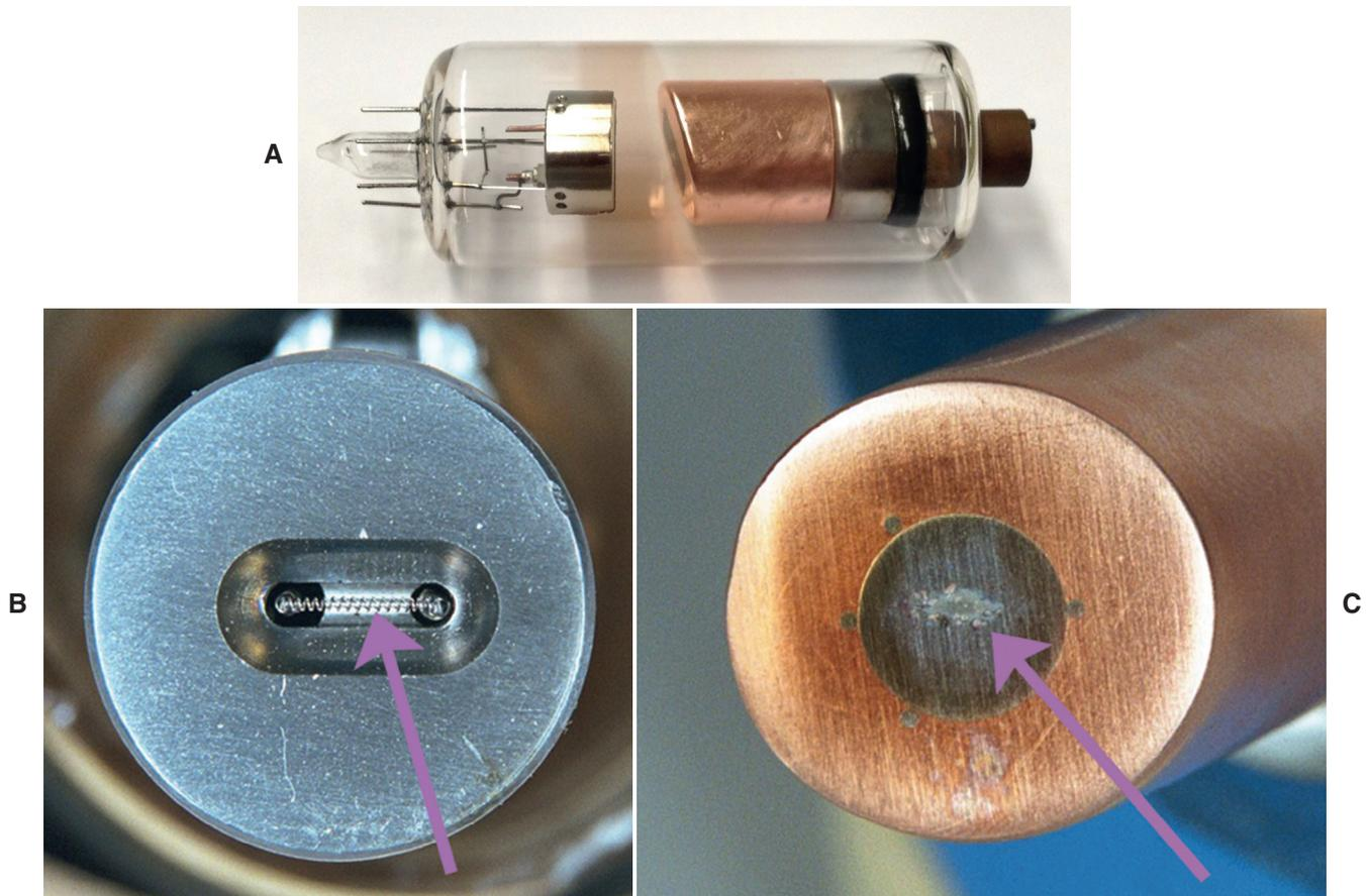
**Fig. 1.7** (A) Dental stationary x-ray tube with cathode on left and copper anode on right. (B) Focusing cup containing a filament (arrow) in the cathode. (C) Copper anode with tungsten inset. Note the elongated actual focal spot area (arrow) on the tungsten target of the anode. (B and C, Courtesy John DeArmond, Tellico Plains, TN.)
