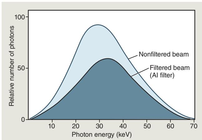
**Fig. 1.18** Spectrum of filtered x-ray beam generated in an x-ray machine showing that an aluminum filter preferentially removes low-energy photons, reducing the beam intensity, while increasing the mean energy of the residual beam. Compare with Figs. 1.15–1.17.
