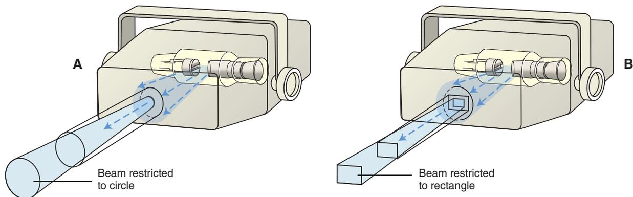
**Fig. 1.19** Collimation of an x-ray beam (blue) is achieved by restricting its useful size. (A) Circular collimator. (B) Rectangular collimator restricts area of exposure to just larger than the detector size and thereby reduces unnecessary patient exposure.
