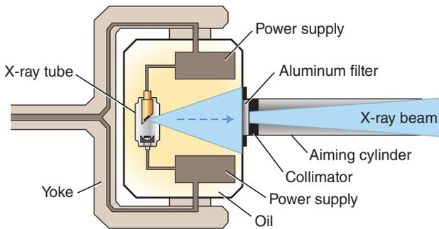
**Fig. 1.5** Tube head showing a recessed x-ray tube, components of the power supply, and oil that conducts heat away from the x-ray tube. Path of useful x-ray beam (blue) from the anode, through the glass wall of the x-ray tube, oil, and finally an aluminum filter. The beam size is restricted by the metal tube housing and collimator. Low-energy photons are preferentially removed by the aluminum filter.
