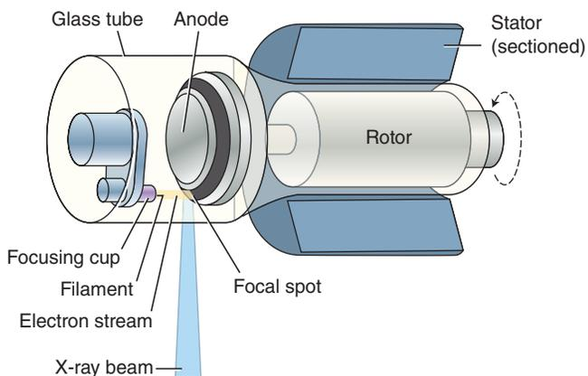
**Fig. 1.9** X-ray tube with a rotating anode allows heat at the focal spot to spread out over a large surface area (dark band). Current applied to the stator induces rapid rotation of the rotor and the anode. The path of the electron beam is shown in yellow, and the useful x-ray beam is shown in blue.
