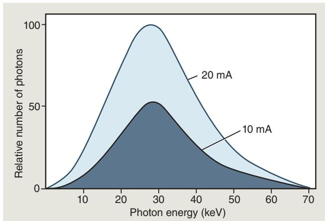
**Fig. 1.16** Spectrum of photon energies generated in an x-ray machine showing that as the mA setting increases (kVp and exposure time held constant), so does the total number of photons. The mean energies and maximal energies of the beams are unchanged. Note similarity to the effect of exposure time; see Fig. 1.15.
