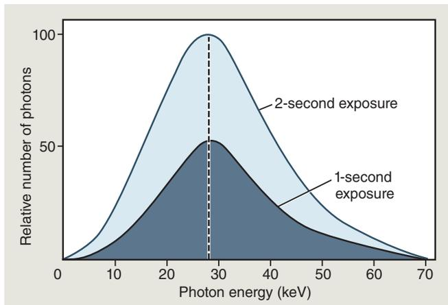
**Fig. 1.15** Spectrum of photon energies generated in an x-ray machine showing that as exposure time increases (kVp and mA settings held constant), so does the total number of photons. The mean energies (dotted line, approximately 29 keV in this example) and maximal energies (70 keV in this example) of the beams are unchanged.
