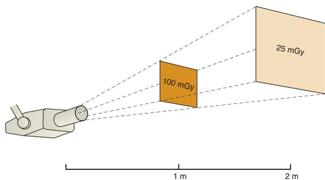
**Fig. 1.20** Intensity of an x-ray beam is inversely proportional to the square of the distance between the source and the point of measure. When the distance from the focal spot is doubled, the intensity of the beam decreases to one quarter.
